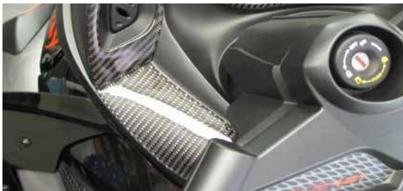
Shown in photo: Adhere Part 11 first, using the pencil line as a guide. Do not try to adhere the part all at once, rather remove the protective backing only from the bottom so you can still maintain alignment of the top without yet adhering it.
