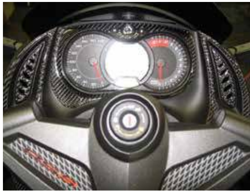
Shown in photo: Use care not to apply 3M adhesive promoter to any section of the dash that will not be covered by the part.
