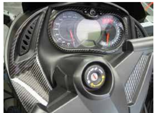
Shown in photo: Remove only the upper protective backing of Part 13 and align it with the lower end of Part 11, then gradually remove the backing while carefully aligning it to the pencil mark.
