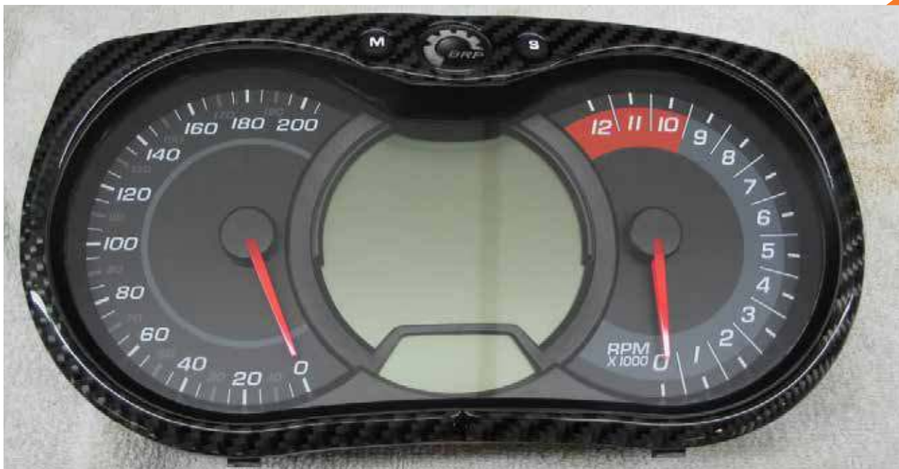
Shown in photo: Peel just enough protective backing to center part over logo & buttons.
