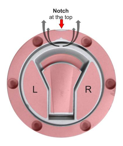
**NOTE:** Outer ring has very tight tolerance due to holes, be sure you are accurately placing the ring in the correct position. **Notch is to be positioned at top center.** Before final placement, open and close gas lid to be sure the gas door has enough space to pivot.
